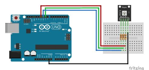
Current has to be limited by using resistors!
